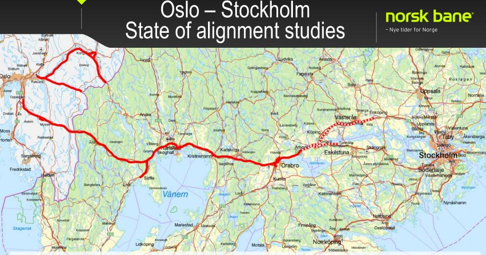
Expected distance Oslo – Stockholm: 500 kms. Current distance: 605 kms. Travel time nonstop 2:00 h. Travel time included 7 – 8 stops: about 2:35 h. 3 - 5 trains per hour and direction, serving 16 – 20 stations. Alternating stops. Freight trains on new line at night, on some sections at day time as well.
