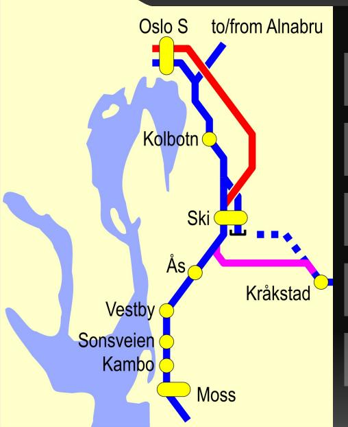
A new, 23 kms long, high speed line for passenger trains only (in red).
